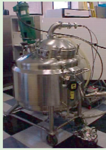
Photo 3: 500-liter pharmaceutical process vessel
