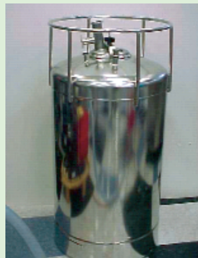
Photo 2: 100-liter pharmaceutical process vessel
