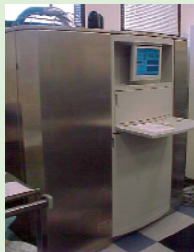
Photo 1: Isodox chlorine dioxide gas generator
