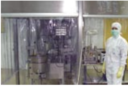
Photo 2: The Acerta DS1 dispensing system as an integrated unit in a fully automated filling line for 1,000–10,000 vials/batch.
