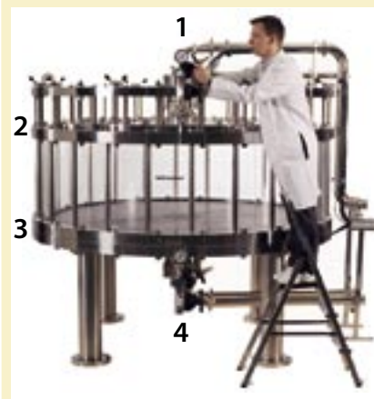
Figure 1: Sampling a column for cleaning evaluation using TOC; 1 (inlet valve), 2 (column gasket), 3 (base gasket), 4 (outlet valve) (WWW.GEHEALTHCARE.COM)
