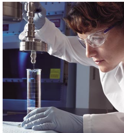
A technician tests the bubble point of a filter membrane. (WWW.MILLIPORE.COM)
