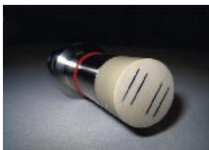
Photo 1: Flush electrode probe developed initially for cell culture and brewing
