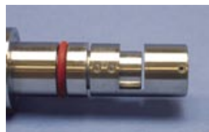
Photo 3: An Ingold probe for fermentation reactors
