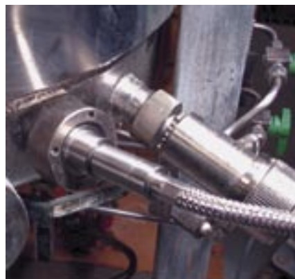
Photo 2: NIR Ingold probe installed in a bioreactor sample port
