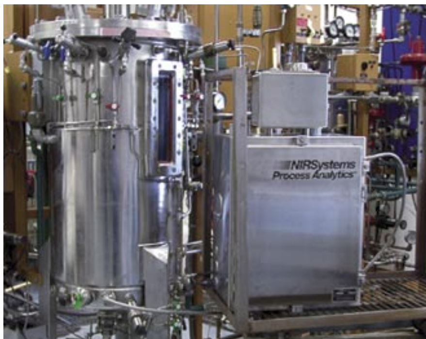
Photo 1: Bioreactor with NIR process instrument
