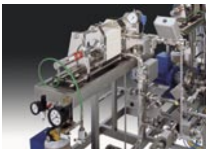
Sartoflow 20 system with hydraulic closure technique for HSA processing (WWW.SARTORIUS.COM)
