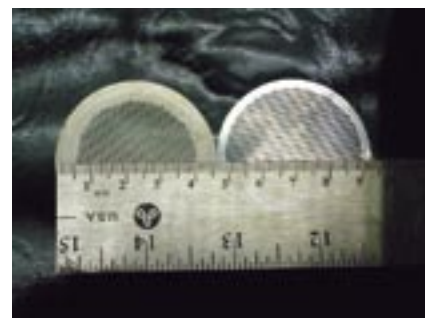
Photo 3: Comparison of support screen perforated area
