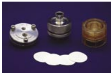
Examples of bench-scale test housings WWW.CUNO.COM
