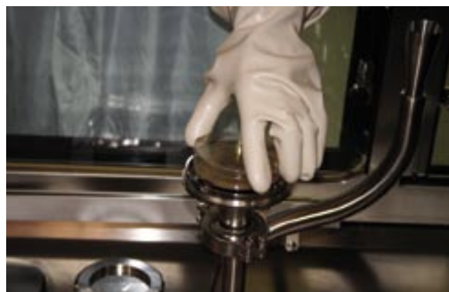
Photo 4: Environmental monitoring (EM) samples can be transferred from the isolator through an IDC beta Biosafe port system.
