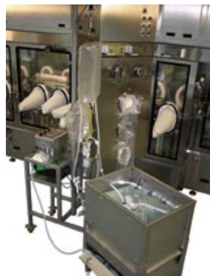
Photo 2: A Flexel 3D bag and Palletank vessel are shown with a transfer set and IDC alpha and beta Biosafe ports docked to the Solvay Pharmaceuticals isolator filling line.
