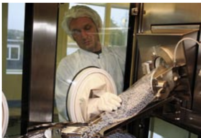
Photo 3: In the Solvay facility, plungers and stoppers arrive gamma-irradiated and contained in a disposable bag that has an IDC beta Biosafe port to dock with the alpha Biosafe on the isolator for aseptic transfer.
