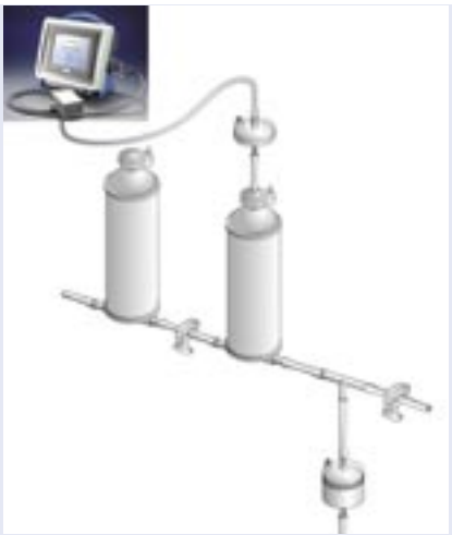
Figure 5: The automatic integrity tester line is attached to the vent filter outlet on the second filter housing.
