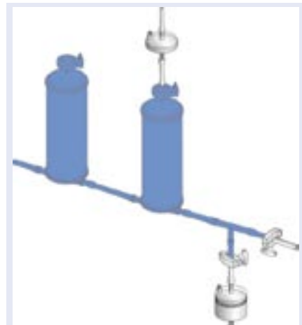
Figure 2: Hydrophobic vent filter prevents ingress of contaminated room air into the area between the first and second filter.
