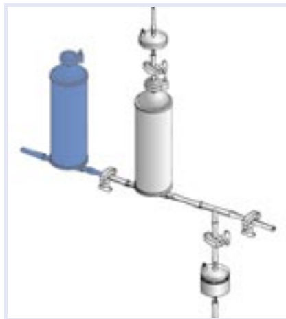
Figure 1: Air is purged from the high-point bleed until a steady flow of liquid with no gas bubbles is observed.
