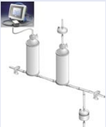
Figure 4: The vent filter upstream of the second filter housing and the line to the barrier filter downstream of the second filter housing are opened.
