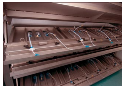
Photo 1: Detail of the Tsunami bioreactor: Because of the different angles of the rocking platforms, only two can be seen in detail. In this configuration, four bags per layer with a culture volume of 35 L each are placed on the platforms, all with air-in and air-out connectors and an inoculation/sampling connector in the middle. Additional connectors are optional. Bags are fixed in place by a slight overpressure; the top left bag is not yet fully inflated in this picture. Total capacity of this model is 16 × 35 L culture volume.
