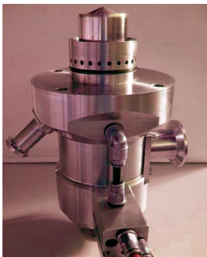
Photo 1: A three-way packing valve removed from its column-head location to show the connections for product, buffer, and slurry lines. The valve is adjusted during operation to allow the column to function in process, packing, or unpacking mode. MILLIPORE CORPORATION (WWW.MILLIPORE.COM)
