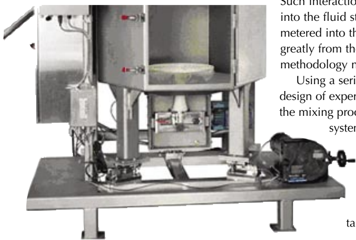
Photo 2: A holding vessel equipped with a side access panel
