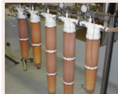
Figure 2: Typical Pall filtration train
